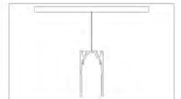
吊灯安装 Chandelier installation
